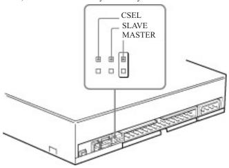
Your computer should have a PRIMARY IDE bus and a SECONDARY IDE bus. Each bus can have one MASTER and one SLAVE device connected to it. Follow the configuration guidlines below for optimum performance and reliability.
